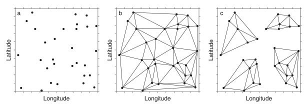
Fig. 3. Principle of clustering with spatial contiguity constraint. (a) Draw the sites on a map. (b) Link the sites by a connection network, here a Delaunay triangulation, which can be represented by an adjacency matrix. (c) Cluster the (univariate or multivariate) community composition response data by agglomerative clustering of *K*-means partitioning, using the link edges as constraints; only adjacent sites or groups of sites can be clustered by the algorithm operating on the response data.
